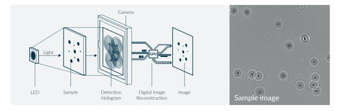
Digital holographic microscopy (DHM) is a state-of-the-art quantitative phase imaging technique that allows automated label-free analysis of cell counts and viability. In DHM, the sample is illuminated with light. As light passes through the sample, some of it
