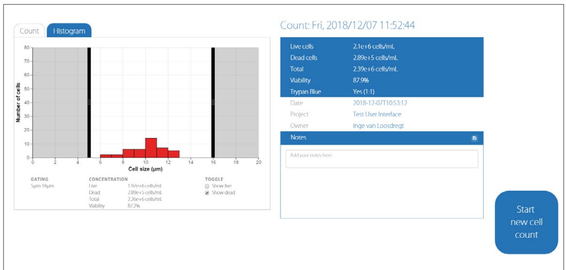
Figure 8. The live cell population is deselected in the toggle box so that only the histogram of the dead cells is displayed.
