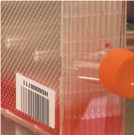
Figure 2. Any liquid inside the flask will distribute evenly into each layer of the flask when it is placed on its side.
