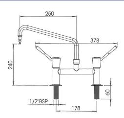
Part No: 910178MIX-W Balanced flow laboratory mixer tap
