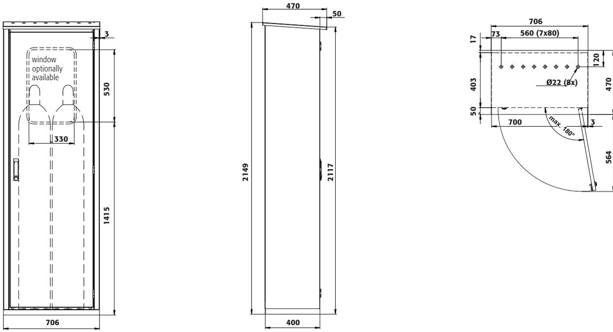
Diagram shows left-hinged door. Dimensions are identical for a right-hinged fitting.
