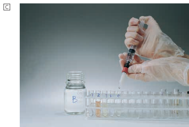
Fig 2. Using StrepTrap HP 1 ml with a syringe. (A) Prepare buffers and sample. Remove the column's top cap and snap off the end. Wash and equilibrate. (B) Load the sample and begin collecting fractions. (C) Elute and continue collecting fractions.
