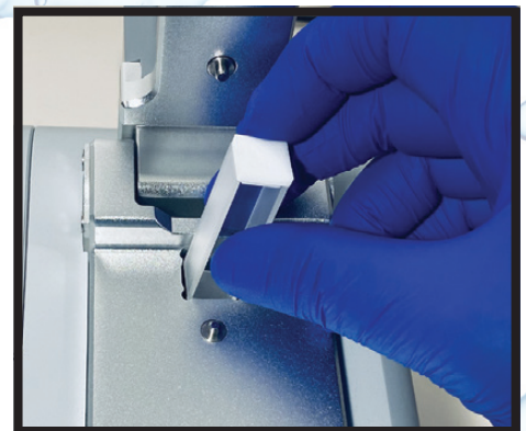
Cuvette port for OD600 readings
