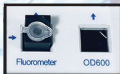
Fluorometer & Cuvette OD600 ports
