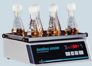
Innova 2000 Maximum flask size: 500 mL Orbit: 1.9 cm (0.75 in)
