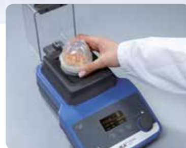
Step 2 | Attach the grinding chamber onto the Tube Mill
