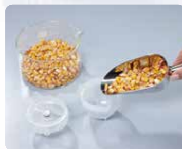
Step 1 | Fill the sample in the grinding chamber
