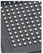
Patented plate carrier using two magnets per well for washing of magnetic bead-based assays
