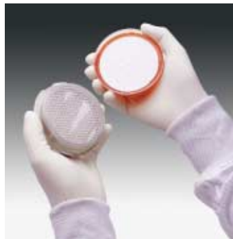
Direct Transfer Method Direct transfer of gelatin membrane to agar plate for fast, accurate detection of microorganisms.
