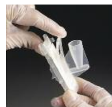
Clip top of funnel and base together.
