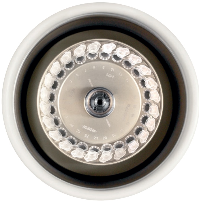
View into the centrifuging chamber showing the 2428 rotor and reaction tubes with open lids
