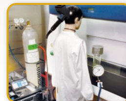
Tracer gas containment test
