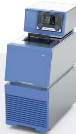
CBC 5 control Refrigerated and heating circulator
