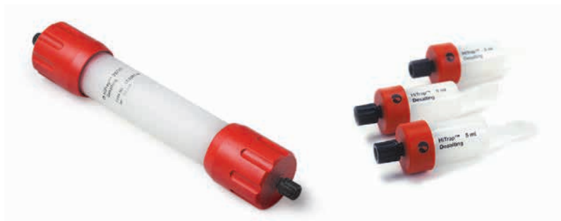
Fig 5.1. Prepacked Sephadex G-25 columns: left HiPrep 26/10 Desalting, right HiTrap Desalting 5 ml.
