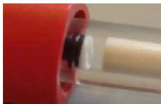
Fig 1.13. The maximum pressure over the packed bed is the maximum pressure the packed bed of chromatography medium can withstand without gap formation. This is not a fixed value.
