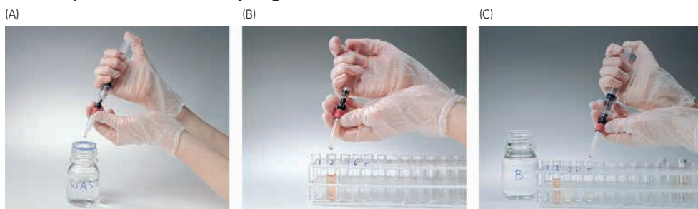
Fig 5.8. Using HiTrap columns with a syringe. (A) Prepare buffers and sample. Remove the column's top cap and twist off the end. (B) Equilibrate the column, load the sample, and begin collecting fractions. (C) Wash and elute, continuing to collect fractions.
