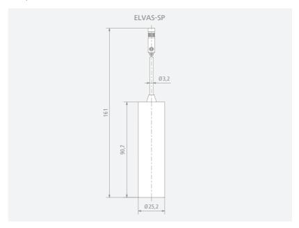
/// Measuring chamber innerdiameters (mm)
