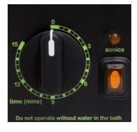
To stop the ultrasonic activity at any time, press the SONICS button while in operation.
