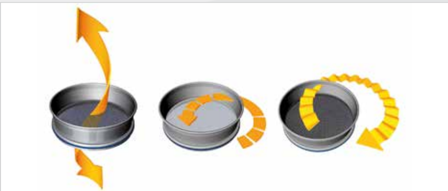
Fig. 2: Principles of 3-dimensional throwing motion (left), horizontal sieving (middle) and tap sieving (right)
