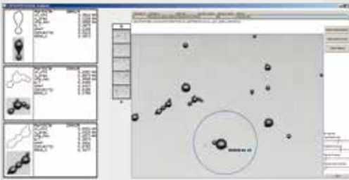
All particle images and corresponding measurement parameters can be optionally stored in the particle library.
