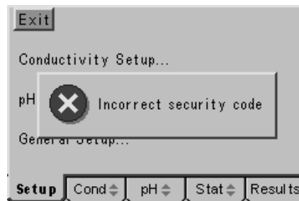
Access to Set Up menus blocked by incorrect security code entry
