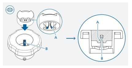
**Note:** When assembling the cover, make sure that the silicone cover is in the correct position.
