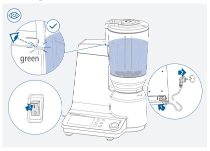
**Note:** After the cover has been securely closed, the color of the LED signal lamp changes from red to green. The unit is only ready for operation when the LED is green.
