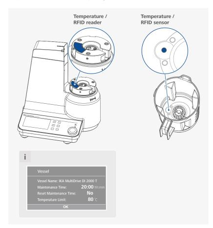
The temperature measurement with the vessel **MultiDrive DI 2000 T** works exclusively with the **MultiDrive control**. When the "Temperature Limit" is set in **MultiDrive control** that the device stops after the temperature is reached. With the setting, both sample and the vessel can be protected from overheating.
