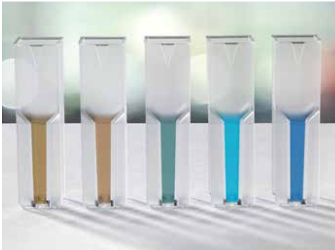
Figure 1: Bradford Protein Assay measured in cuvettes, showing increasing protein concentrations.
