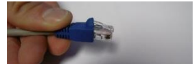
Slide boot back over lock clip
