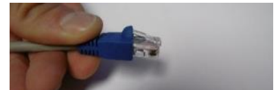
Slide boot back over lock clip
