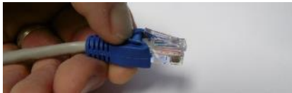
Pull boot back to access lock clip
