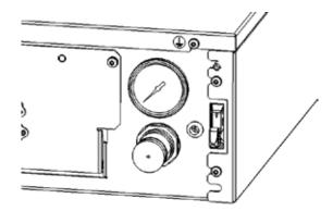
Adjust the gauge to the required pressure. To ensure a smooth pressure profile, it is not recommended to increase the output pressure to above the factory set 116psi.
