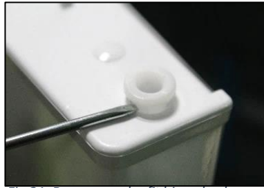
Fig 21. Remove and refit hinge bush
