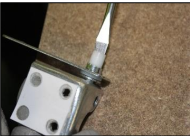
Fig 15. Rotate and fit hinge
