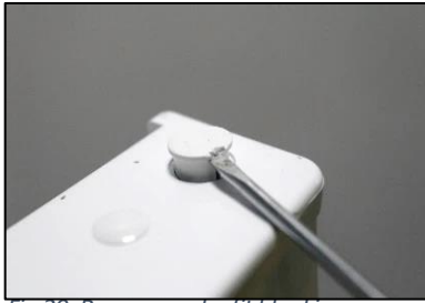
Fig 20. Remove and refit blanking cap
