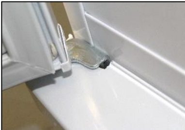
Fig 25. Refit foot plate
