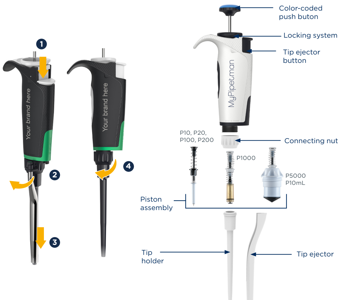
Figure 11 MyPIPETMAN® piston assembly (disassembled)
