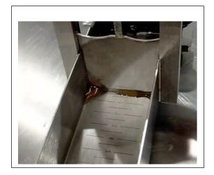
Our Bostwick Consistometers are manufactured in accordance with ASTM Standard, Designation: F1080 – 93 (Reapproved 2008).
