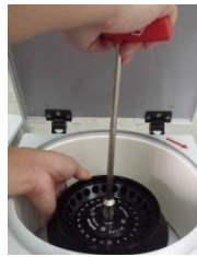
Tool for rotor with nut
