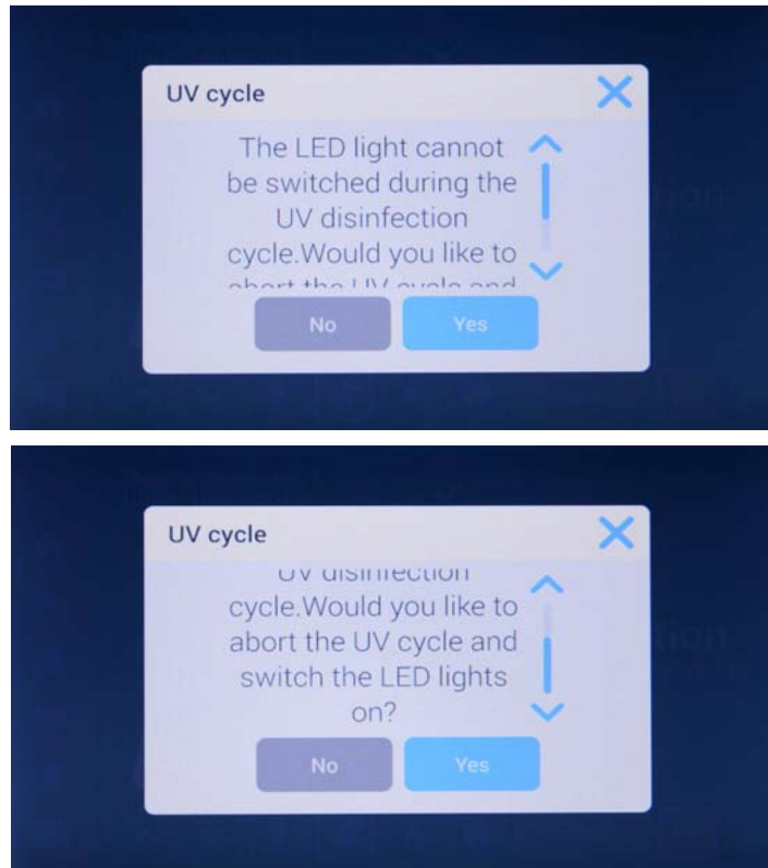
Figure 44 UV Cycle Alert When Light Bulb Button is Tapped During UV Disinfection
