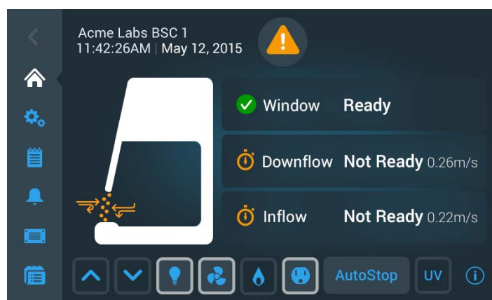
Figure 32 Main Screen - Unit Starting Up
