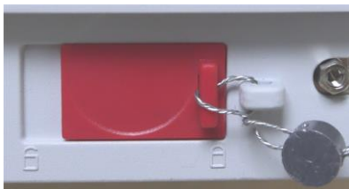
Locked with Wire Seal
