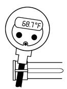
Insert the probe into the "loop" on the cover. It makes a perfect holder.
